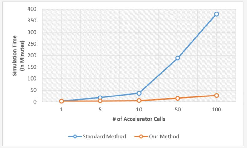
Simulation time of TE using different # of Accelerator calls
