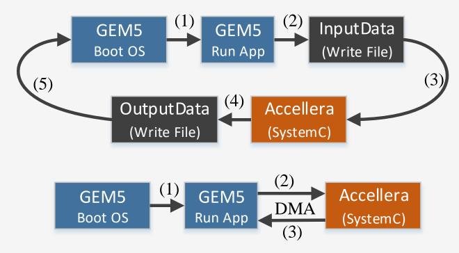
(i) Standard (top) & (ii) Our novel method integrating GEM5 Full System Simulator with Accellera Simulator
