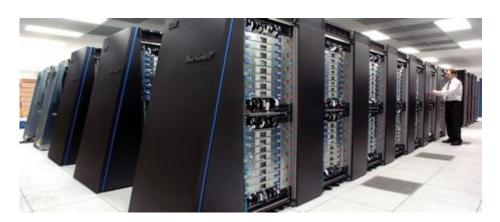
The IBM Blue Gene/P supercomputer "Intrepid" at Argonne National Laboratory runs 164,000 processor cores in 40 racks/cabinets connected by a high-speed 3-D torus network.
